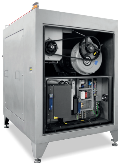
The electrical panel is embedded into the machine cabinet. The electrical panel can swing away in order to grant full access to the interior of the machine for maintenance etc.
