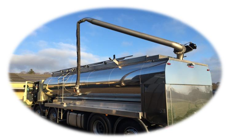
The lifting pipe reduces the weight on the feeding tube. This reduces the load on the driver and provides and easier and better workflow.
